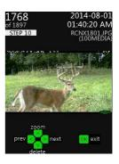
Play Videos – When you select this option, the camera will enter into a slide show function to view thumbnails of the videos on the memory card. The LEFT and RIGHT directional buttons will allow you to scroll through the thumbnails. The UP directional button will play the video while the DOWN directional button will allow you to delete the video being viewed at that time. Pressing the OK button will allow you to exit from the video slide show and return you to the Home page.
