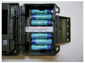
**Warning!** Do not mix battery types! Damage to the camera can result and your warranty will be voided if you mix battery types.
