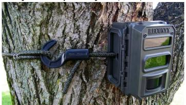
We recommend that you mount your camera at a height of approximately 4 feet. This height is optimal for detecting animals in the field of view of the camera as well as for accessing the camera's card, batteries, and controls.
