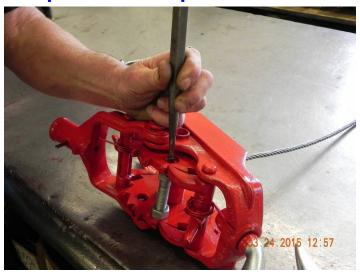
After rivet is peened down, remove bolt.
