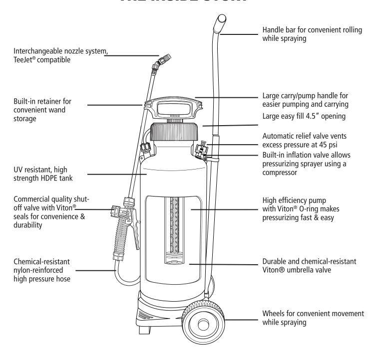
Chemical resistant Viton® seals in key locations withstand harsh chemicals for long service and durability. Includes 4 Nozzles to Meet Virtually Every Spraying Need. Accepts TeeJet® nozzle tips.
