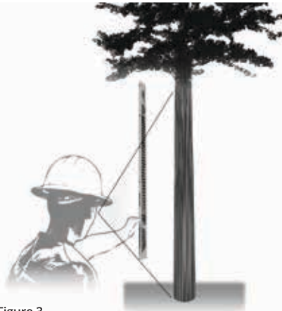
Figure 3 Stick is 25" from eye and 66' from tree. Top measurement is point tree is topped; bottom is point tree is severed at stump. This tree contains three 16' logs.
