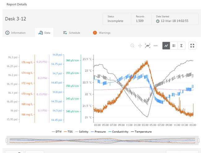
If compensating for Depth to Water enter your depth to water reference measurement and the date/time the measurement was taken (typically taken with a water level indicator before data is uploaded from the sensor) before clicking Continue.
