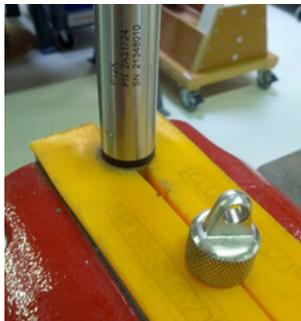
*Cableless Sensor—gripping on knurled area*
