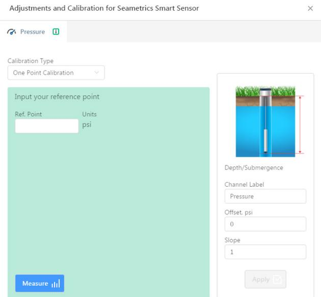
Aqua4Plus 2.0 will take 10 readings and display the average. Watch for stability while Aqua4Plus 2.0 is measuring to ensure an accurate calibration.
