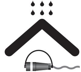
**Do install sensor so the connector end is kept dry**
