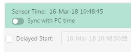
Check the Delayed Start box and enter the desired date/ time you would like logging to start. This is useful for syncing data when setting up multiple sensors on a site. Data will start logging at the set date/time rather than immediately when Start is pressed.
