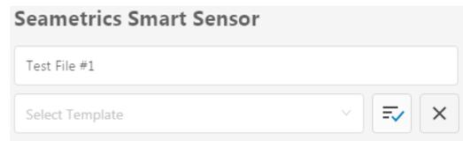
The 3 previous Logging Schedules that were programmed to a sensor will be listed under the Select Template drop down menu. There you will also find pre-programmed logging schedules such as 24 hour pump test, along with any custom logging schedules saved by the user.
