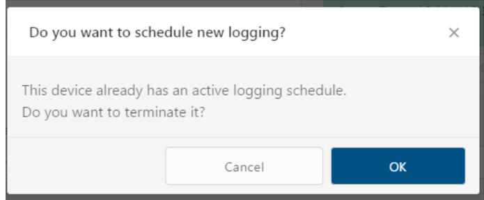
Starting a new file will automatically terminate the active logging and begin the new logging schedule. Real-time data is available during active logging.
