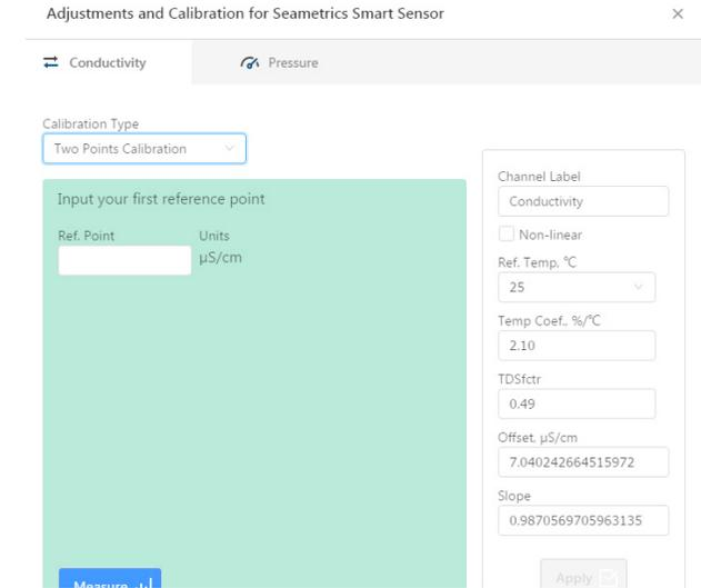
The calibration screen will default to the conductivity channel, you may also switch to the Pressure channel if you need to perform a pressure calibration setup.
