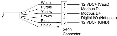
*For Modbus® with firmware lower than 2.0
