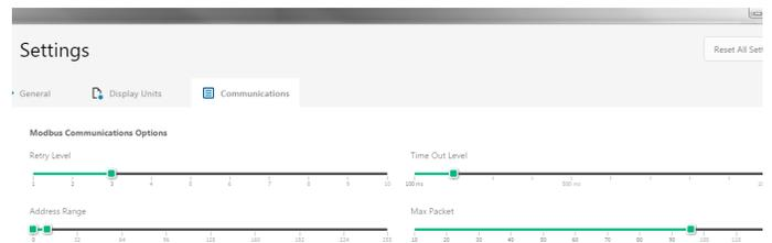
Under the Communications tab you can change your Modbus communication settings. Typically you will only need to change the address range to connect to sensors outside of Modbus address 1-10. In certain cases we may need to change the Retry and Timeout settings to overcome communication issues on very long, or corroded cabling. See Troubleshooting section or contact Seametrics Tech Support for details.
