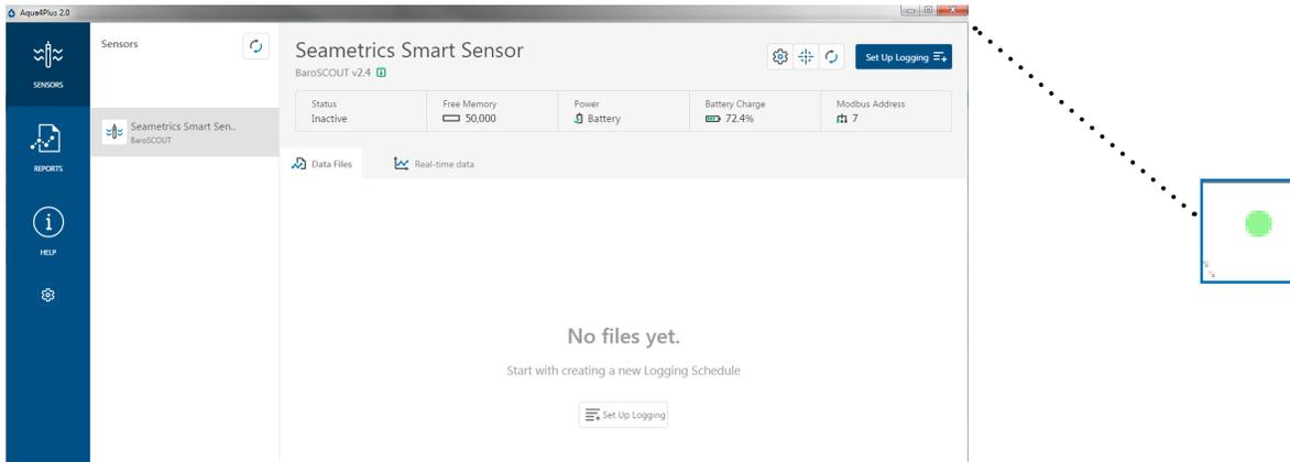
If your sensor still won't connect you can expand the Modbus address range under program settings here:
