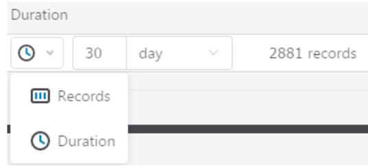
When set by number of records the time of the recording phase will be displayed detailing how long that phase will run. When set by time, the total number of records for that phase will be displayed.
