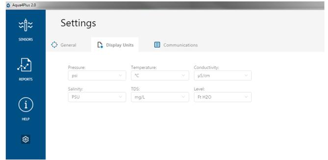
Under the Display Units tab you can select your desired display units for the supported channels. These may be changed at any time and associated Real-Time readings and Reports will rescale to the currently selected display unit. To change Direct Read units scaling see Sensor Settings.
