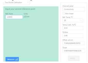
Aqua4Plus 2.0 will take 10 readings and display the average. Watch for stability while Aqua4Plus 2.0 is measuring to ensure an accurate calibration. To accept the first point reading click Ok.
