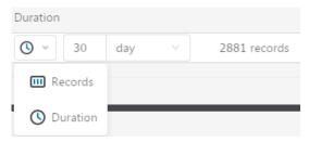
When set by number of records the time of the recording phase will be displayed detailing how long that phase will run. When set by time, the total number of records for that phase will be displayed.
