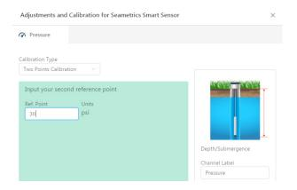
Aqua4Plus 2.0 will take 10 measurements and display the average. Watch for stability while Aqua4Plus 2.0 is measuring to ensure an accurate calibration.
