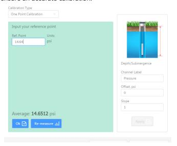
Click Ok to accept the reading and Aqua4Plus 2.0 will calculate a new pressure offset. Click Apply to confirm the new offset value and Aqua4Plus 2.0 will provide a real time reading to verify calibration was successful:
