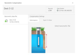
If compensating for Depth to Water enter your depth to water reference measurement and the date/time the measurement was taken (typically taken with a water level indicator before data is uploaded from the sensor) before clicking Continue.
