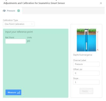
Click Apply to confirm settings and Aqua4Plus 2.0 will provide a real time reading to confirm.
