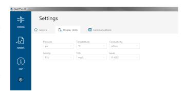
Under the Display Units tab you can select your desired display units for the supported channels. These may be changed at any time and associated Real-Time readings and Reports will rescale to the currently selected display unit. To change Direct Read units scaling see Sensor Settings.
