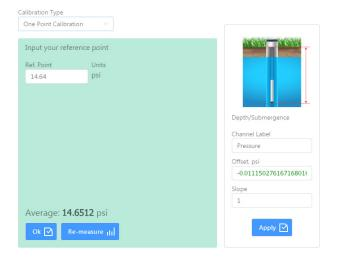
2 Point submergence calibration **ONLY RECOMMENDED IF YOU HAVE AN ACCURATE PRESSURE REFERENCE**. Our Smart Sensors rarely change slope during normal use, however if you have an accurate pressure source it is possible to perform a 2 point calibration on the pressure channel.
