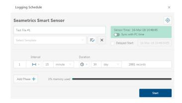
Click to switch between interval and continuous data recording (supported sensors only) Select your continuous rate from the drop down box here.
