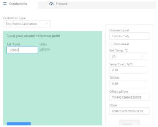
Aqua4Plus 2.0 will take 10 readings and display the average. Watch for stability while Aqua4Plus 2.0 is measuring to ensure an accurate calibration. To accept the second point reading click Ok. Your new offset and slope values will appear to the right, confirm other settings as needed and click Apply to confirm your new slope and offset values. Aqua4Plus 2.0 will provide a real time reading to verify calibration was successful.
