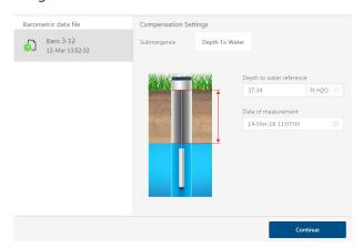
Aqua4Plus 2.0 will perform the barometric compensation and create a new compensated report. Original reports are retained as uploaded.
