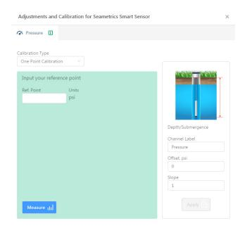
Aqua4Plus 2.0 will take 10 readings and display the average. Watch for stability while Aqua4Plus 2.0 is measuring to ensure an accurate calibration.
