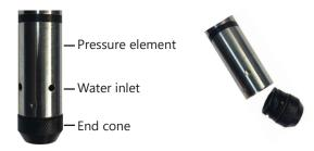
Gently twist off the end cone and carefully remove debris
