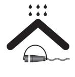
Do install sensor so the connector end is kept dry
