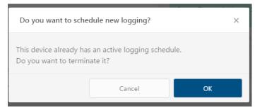
Starting a new file will automatically terminate the active logging and begin the new logging schedule. Real-time data is available during active logging.
