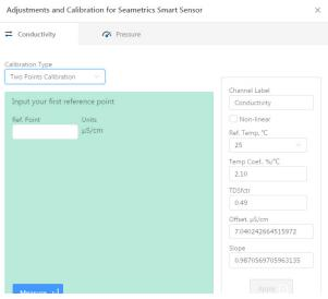
The calibration screen will default to the conductivity channel, you may also switch to the Pressure channel if you need to perform a pressure calibration setup.
