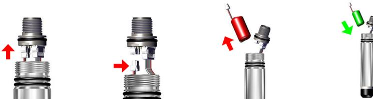
Before sealing the housing back up, replace the O-ring on the connector insert with the one provided. To reinstall the connector insert push it straight back into the housing noting the two flats on the insert as well as inside the housing. These flats prevent the connector insert from rotating during normal use and must be properly keyed when re-installing the insert for the retaining clip to seat properly.
