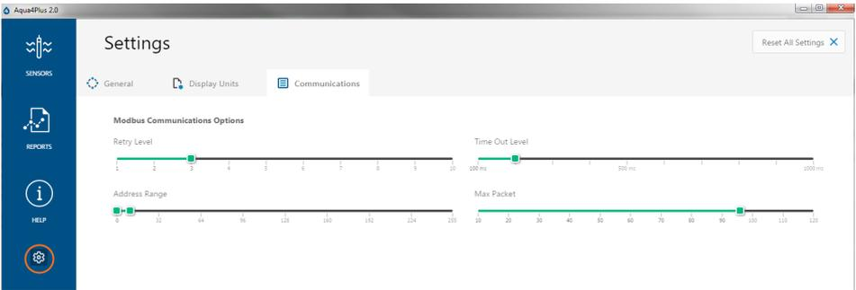
Simply drag the Address Range slider higher up to increase the maximum Modbus address scanned. If you've scanned all the way up through address 255 and still have no connection click Troubleshooting for further troubleshooting or contact Seametrics Tech Support for assistance.
