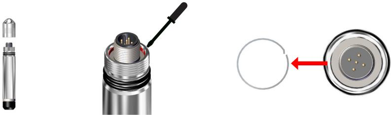
Next, remove the connector insert by carefully pulling straight up while working it side-to-side to help break the O-ring seal. You don't want to pull too hard causing the O-ring seal to release suddenly as that could damage the internal wiring. There is roughly  $\frac{1}{2}$ " of slack in the internal wiring. Once the insert has been removed from the main housing you can disconnect the battery pack.
