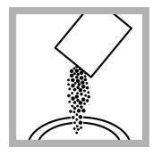
9. Add one 25-mL DPD Free Chlorine Reagent Powder Pillow or one 25-mL DPD Total Chlorine Reagent Powder Pillow to the second sample cell.
