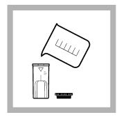
2. Prepare the blank: Fill a 1-cm/10-mL sample cell to the 5-mL mark with sample. Close the sample cell.
