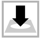
**4.** Insert the blank into the cell holder. Point the triangle mark on the sample cell away from the keypad.
