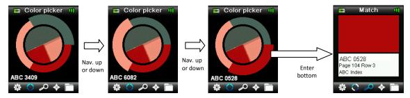
4. Select the desired color by pressing **Enter** to display details of the match.
