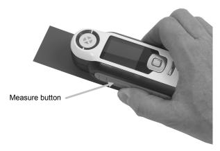
Horizontal, vertical, and angled orientations are acceptable as long as the instrument makes good contact with the sample.
