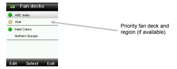
4. Select the fan deck settings option from the list by pressing the up and down sides of the **Navigation** control.
