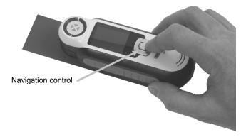
Depending on the fan deck selected, additional information associated to the color can be displayed and selected using the Navigation control.
