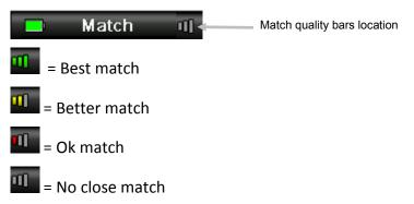
The bars are for informational purpose only. Three "green" bars is the best possible match, where as one "red" or two "yellow" bars indication basically informs you that instrument made a suitable match. The fewer color bars on a measurement, the more likely color differences will be noticed.
