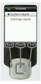
Screens that contain images of "arrows" indicate that the Up and Down sides of the Navigation control are used to adjust or page-through options and colors.
