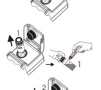
Open the instrument lid, slightly rotate the cuvette and take a new reading.
