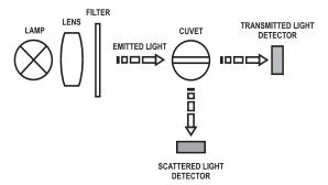
The optical system and measuring technique alow the compensation of lamp intensity fluctuations, minimizing the need of frequent calibration.
