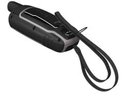
2 Thread the other end of the strap through the loop, and pull it tight.
