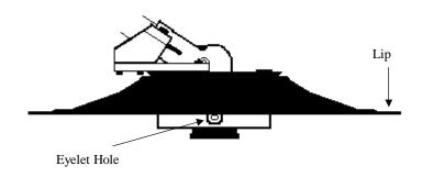
If the eyelet hole is inside the disk slightly, place a metal washer under string head to move string outward. If the eyelet hole is more than an 1/8" beyond the lip your trimmer may cut a wider edge than desired. A spacer between the gearbox and the EDGIT may be required to place the EDGIT's lip adjacent to the spinning string plane.
