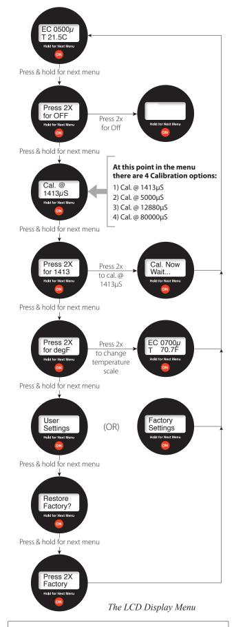
Note: To change the temperature scale between °C and °F, press and hold the ON button repeatedly until "Press 2X for degF" displays. Press the ON button 2 times quickly to change the scale.
