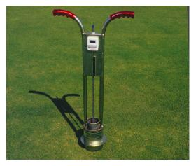
Turf-Tec finally has answered the age old question, "How do I determine Infiltration rate?" The Turf-Tec Infiltrometer is simple to operate and easy to use! Determine infiltration rate in as little as fifteen minutes.
