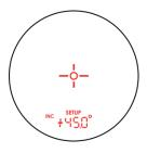
Tilt the laser to the desired angle and press .
