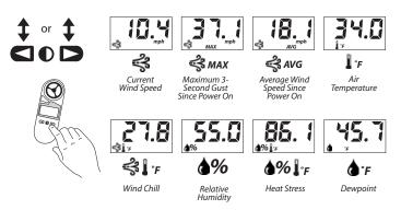
4) Select the units of measure. Press ▶ while holding ● to scroll through the units of measure.
