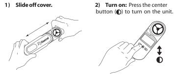
Select operating mode. Press the right arrow (▶) to scroll through the measurements listed below. Press the left arrow (◄) to scroll through the measurements in reverse order. The instantaneous measurements will be displayed. (See Understanding the Measurements section for more information.)
